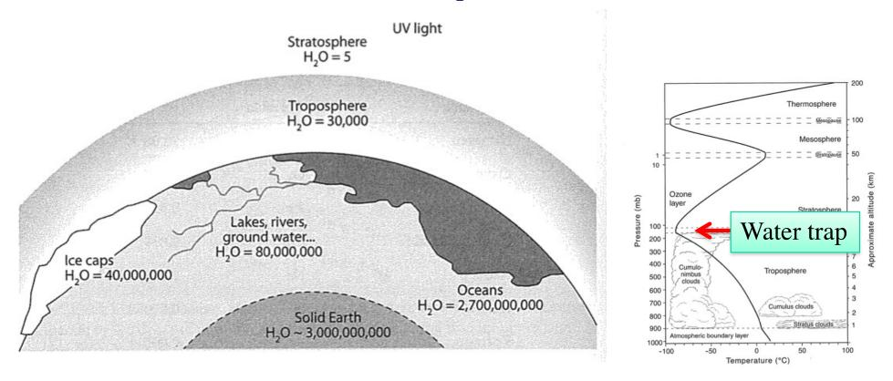
Thanks to the negative temperature gradient in the troposphere, all water precipitates in the higher tropospheric layers (due to Clausius-Clapeyron), and none migrates to the upper atmosphere
