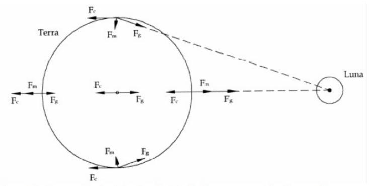
Surface tides can be estimated by calculating the vectorial sum of the centrifugal force and the gravitational force (with its gradient inside the planet or satellite)
