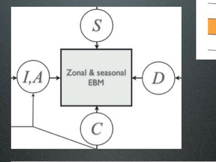
$$I_i + C_i \frac{\partial T}{\partial t} - \frac{\partial}{\partial x} \left[ D_i \left( 1 - x^2 \right) \frac{\partial T}{\partial x} \right] = S_i$$
