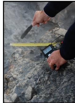
Sampling in Pool 2 hot spring sediment (pH 1.5, 92°C)
