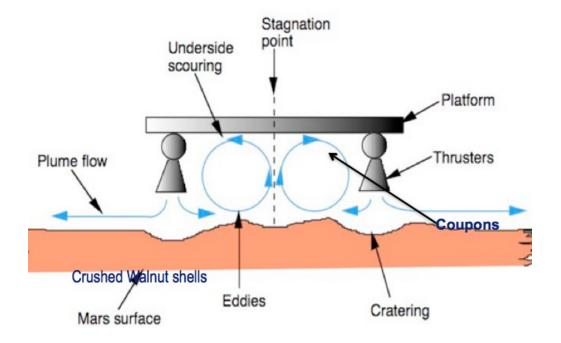
Different planetary protection cleanliness levels for different parts of a spacecraft do not necessarily prevent soil contamination because these cleaning strategies evolved without consideration of the effects of the descent engine plumes.
