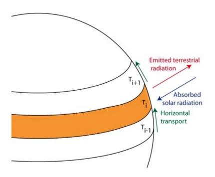
$$I_i + C_i \frac{\partial T}{\partial t} - \frac{\partial}{\partial x} \left[ D_i (1 - x^2) \frac{\partial T}{\partial x} \right] = S_i (1 - A_i)$$
